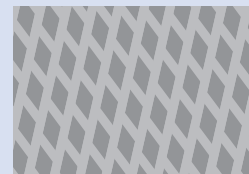
Diamond-shaped lubricant reservoirs
