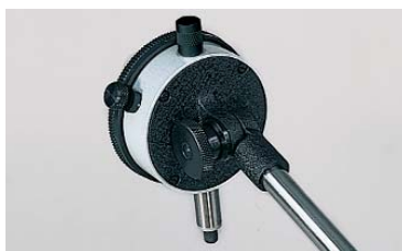
Clamp mechanism grips indicator lug back.
