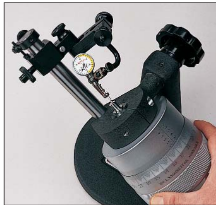
Dial test indicator is held in place by an offset attachment.
