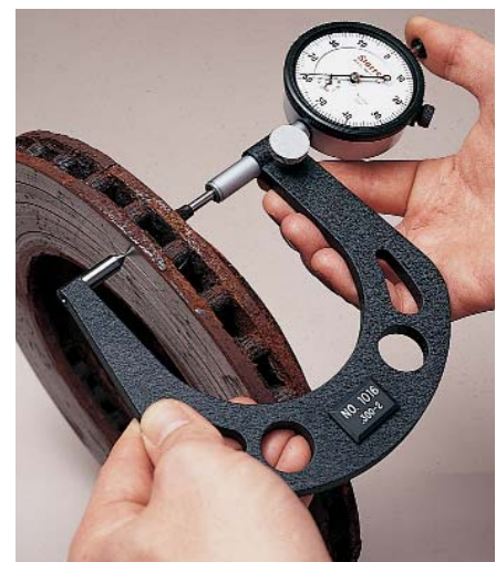
Measuring the groove depth of a disc brake rotor with the No. 1016.
